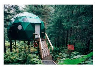
arranged in a spherical shape, giving it an incredibly strong structure with very little construction material needed. It consists of the hub, struts, plywood, dormers, extensions, and skylights. These homes are also very energy efficient. They are unique looking and can be built relatively inexpensively compared to a traditional home. A dome home, a kit for a 40-foot in diameter, was \$30,000.
